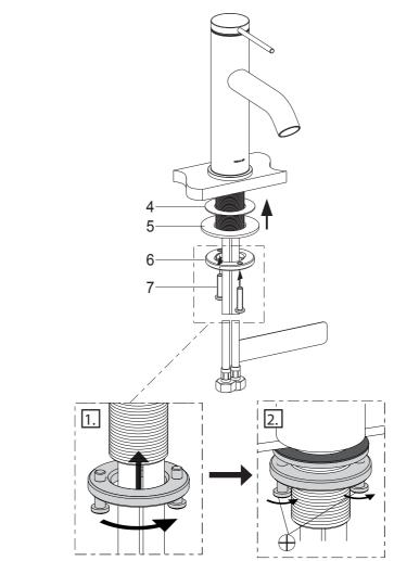
Position the faucet, install the screws(7) into the mounting nut(6). From underside of the lavatory, place the washers(4, 5) onto the shank. Tighten the mounting nut to secure the faucet. Tighten the screws.
