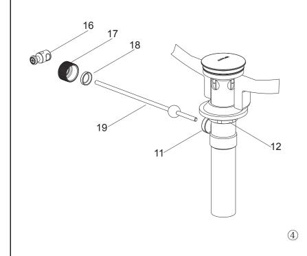
Remove the latch(16) and retaining nut(17). Fit the plastic washer(18) and retaining nut onto the ball lever(19). Insert the ball lever assembly into the drain lever hole and through the stopper hole. Tighten the retaining nut.
